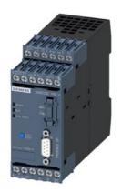
Basic unit SIMOCODE pro V PB PROFIBUS DP interface 12 Mbit/s, RS 485, 4l/3O freely parameterizable, Us: 110...240 V AC/DC, input for thermistor connection Monostable relay outputs, expandable by extension modules
