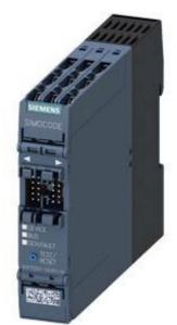
Basic unit SIMOCODE pro S, PROFIBUS DP interface 1.5 Mbit/s, 4I/2O freely parameterizable, Us: 110...240 V AC/DC, input for thermistor connection Monostable relay outputs, expandable by a multifunctional module
