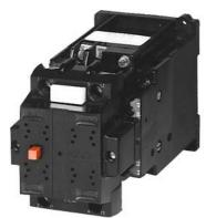
Contactor, Size 2, 2-pole, DC-3 and 5, 32 A Auxiliary contacts 22 (2 NO + 2 NC) 110V DC DC operation
