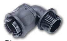
90° sharp edge fixed male connector with plastic thread made of high quality, halogen free and flame retardant polyamide. It ensures high resistance to traction and torque and good mechanical and thermal performances. It's the ideal solution for static and dynamic applications and for most environments. With connectors and gaskets, it provides a protection index IP68.
