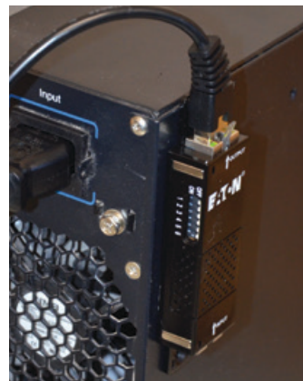
Eaton EMP Gen 2 installed
